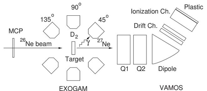
FIG. 1: Experimental setup in the VAMOS vault.
