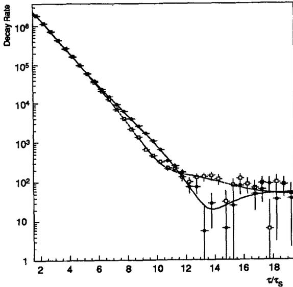
Fig. 1. Acceptance-corrected decay rate of  $K^0(\square)$  and  $\bar{K}^0(\bullet)$  into  $\pi^+\pi^-$ . The lines are the expected rates (Eq. (1)) when the PDG-94 values are used for  $\Delta m$ ,  $\tau_S$ ,  $\tau_L$  and  $\eta_{+-}$ .
