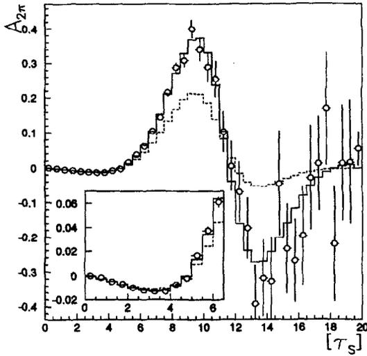
Fig. 2. Asymmetry  $A_{2\pi}$  as a function of the decay eigentime. The dots represent the CPLEAR data on  $\pi^+\pi^-$  decays. The inset displays the data at short decay times. The solid line is the result of our fit. The dashed line represents  $A_{2\pi}$  with positive values of  $\alpha, \beta, \gamma$  which are for illustration 10 times larger than the actual limits obtained (Eq. (11)). The shape of the curve is insensitive to the value of the parameter  $\gamma$ .
