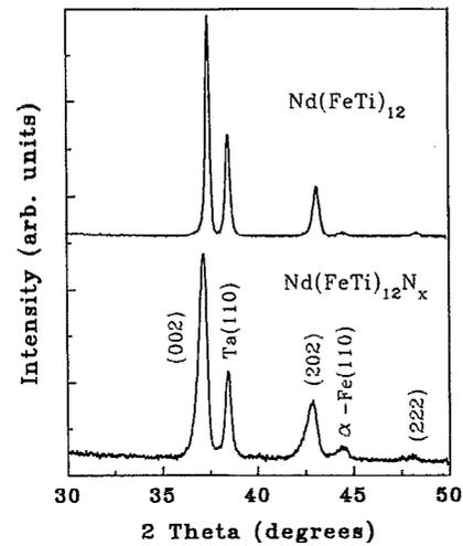
FIG. 2. X-ray diffraction patterns of a  $\text{Nd}(\text{FeTi})_{12}$  film and a  $\text{Nd}(\text{FeTi})_{12}\text{N}_x$  film of about 1 μm thick on Ta substrates.
