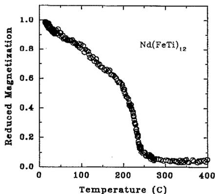
FIG. 5. Thermal-magnetization curve for a  $\text{Nd}(\text{FeTi})_{12}$  sample. The field was about 500 Oe and temperature changing rate was about  $20^\circ$  per minute.
