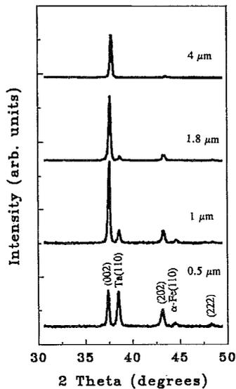
FIG. 1. X-ray diffraction patterns of  $\text{Nd}(\text{FeTi})_{12}$  films with different thicknesses on Ta substrates. The deposition conditions are an argon pressure of 1.5 mTorr, a power of 100 W, and a substrate temperature of 390 °C.
