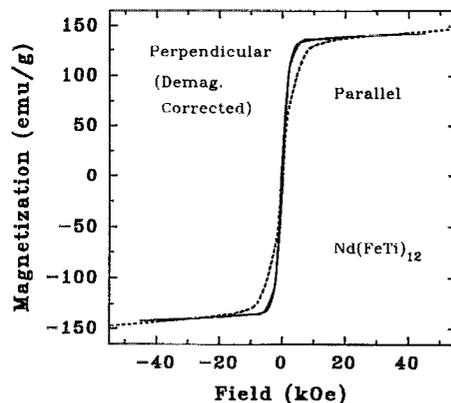
FIG. 3. Hysteresis loops of a  $\text{Nd}(\text{FeTi})_{12}$  film of about 1 μm thick measured at room temperature. The perpendicular loop has been corrected for demagnetization.
