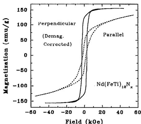
FIG. 4. Hysteresis loops of a  $\text{Nd}(\text{FeTi})_{12}\text{N}_x$  film of about  $1\ \mu\text{m}$  thick measured at room temperature. The perpendicular loop has been corrected for demagnetization.
