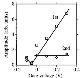
FIG. 2. Harmonic content of CO for sample 3A in forward bias. Squares - 1st harmonic, diamonds - 2nd harmonic. Lines are drawn to guide the eye.
