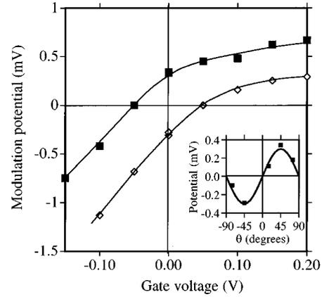
FIG. 1. Amplitudes of fundamental potential component for sample 1 plotted against gate voltage. Squares - sample 1A, diamonds - sample 1B. The lines drawn are to guide the eye. Inset - amplitudes plotted against orientation angle. The solid line is the predicted fit with an amplitude of 0.3 mV.
