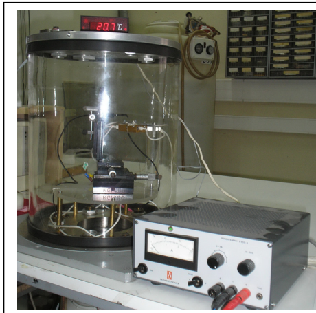
Fig. 2.7: (a) Measurements system, (b) probe station, (c) Temperature-controller system (d) Samples ( \text{Pt/CeO}_2/\text{p-Ge} ) on gold-plated chuck.
