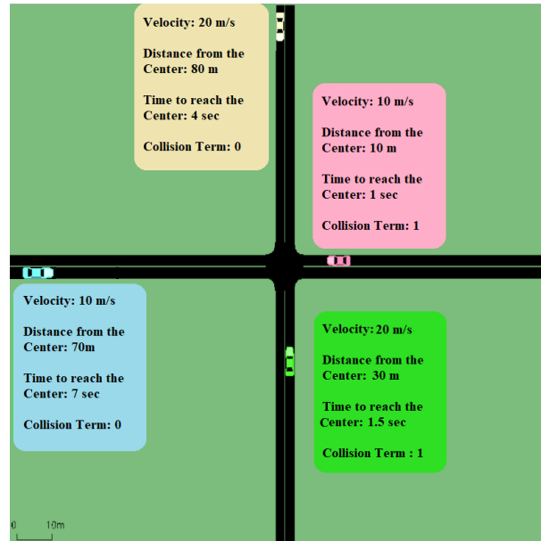
Figure 4.1: An example of how the collision term is calculated.
