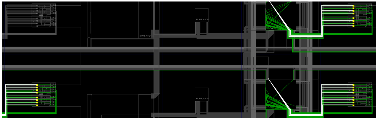
Figure 2.27: Part of the Ring Oscillators, seen to utilize lookup tables
