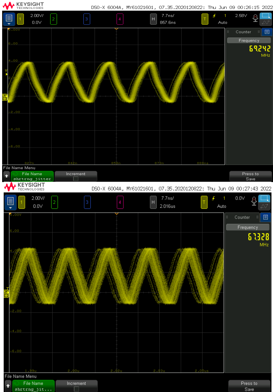
Figure 3.1: The waveform after 50 (top) and 70 (bottom) oscillations
