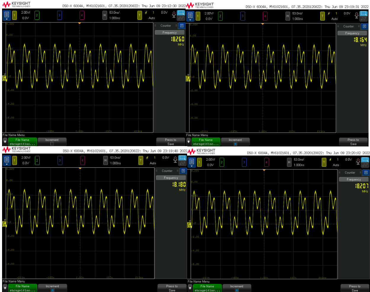
Figure 2.36 : Frequency from Rings of Length 161
