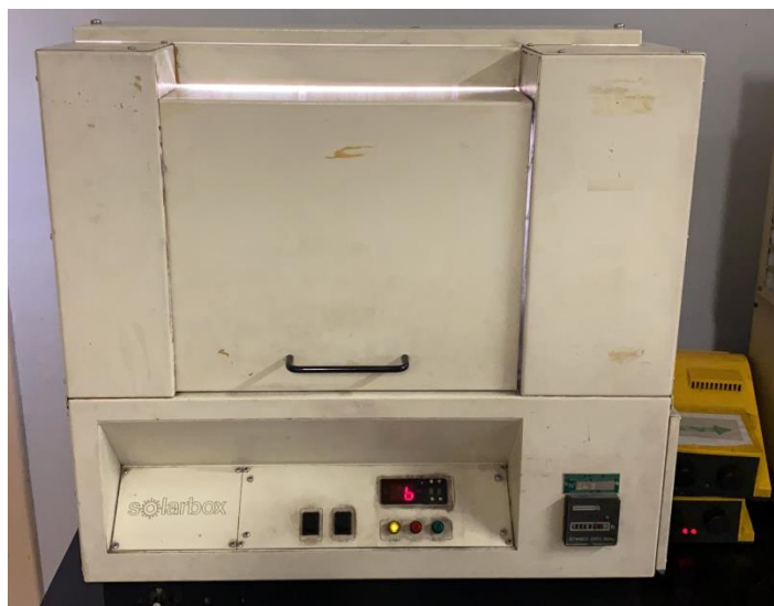
Figure 6.2. Sunlight simulator used during my secondment at the University of Turin.
