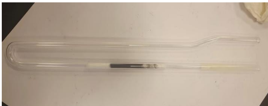
Figure 5.12. Photograph of the reactor after the \text{H}_2\text{S} adsorption experiments: elemental sulfur is visible on the right near the exit
