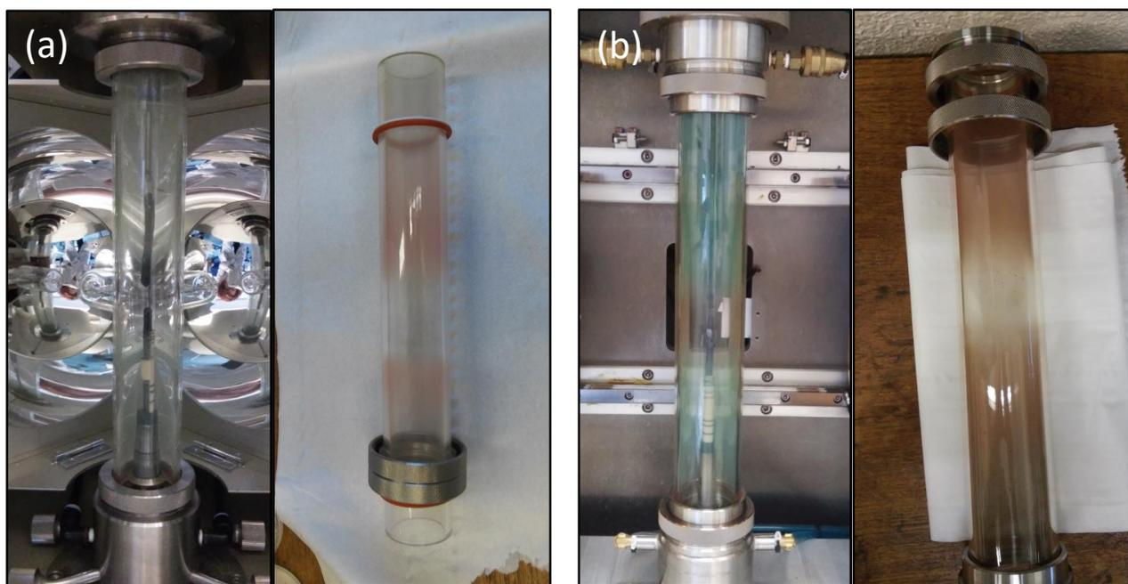
Figure 3-14 (a) Coated quartz tube after the first #1 growth attempt using  $\beta\text{-NaMnO}_2$  as starting powder. (b) Coated quartz tube after the #5 growth attempt using  $\beta\text{-NaMnO}_2$  as starting powder which resulted in crystal boule of  $\text{Na}_{0.7}\text{MnO}_2$
