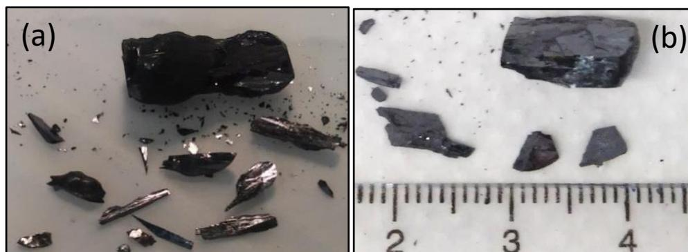
Figure 3-13 Crystal boules grown using beta polymorph as starting powder. Several crystal flakes could only be separated after crushing the as grown boule.
