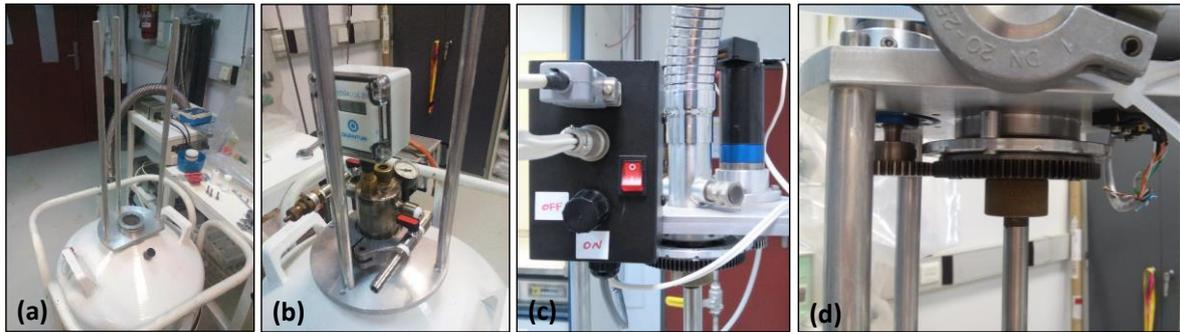
Figure 8-9 (a) Base of the cryogenic liquid transfer line, (b) Liquid N<sub>2</sub> level indicator, (c) Control circuit in box with DC motor, (d) Gear transmission system with metal stopper rod that changes the condition of the two micro switches.
