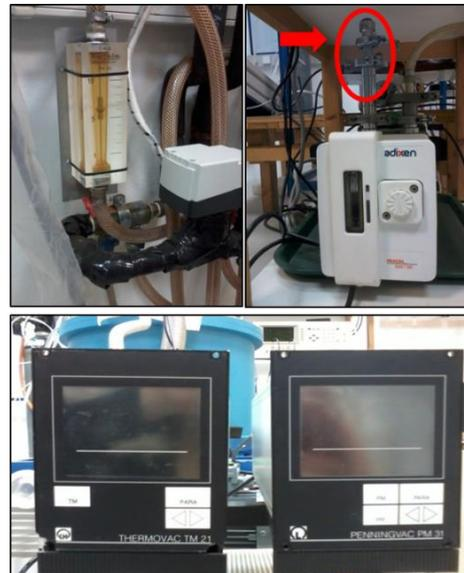
Fig.5 **top-left:** water flow meter, **top right:** rotary vacuum pump for low vacuum **Bottom:** vacuum gauges and controller of the turbo pump
