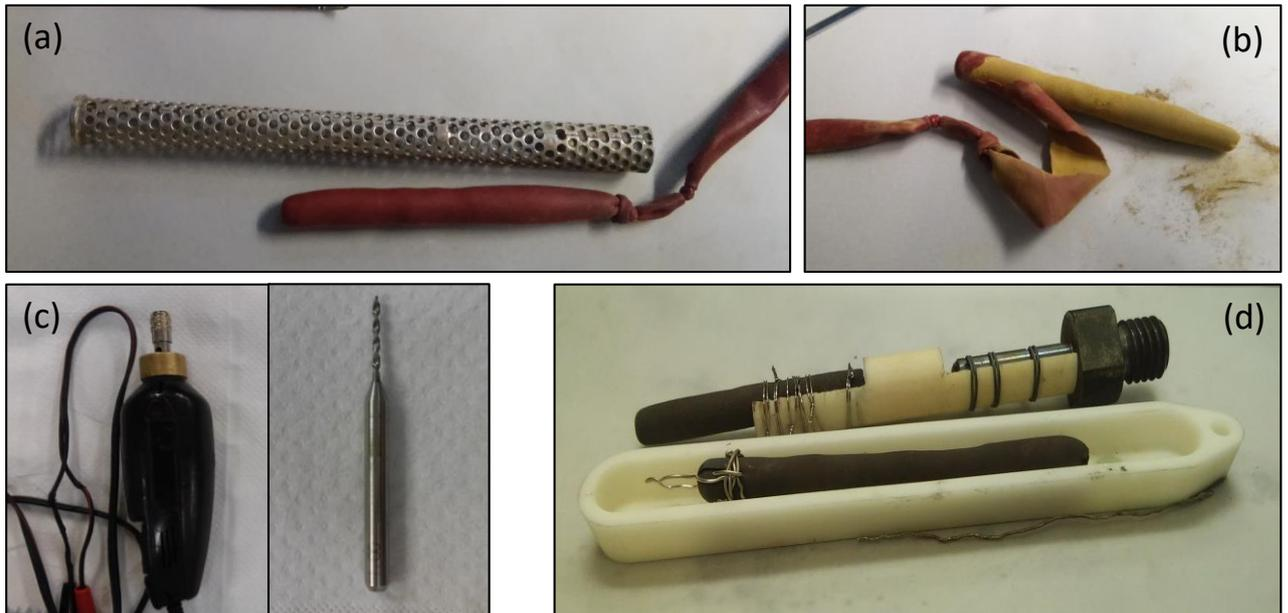
Figure 3-8 (a) Shape powder in a cylindrical rod by hand pressing it inside a ballon (b) cut-reveal the rod after being isostatically pressed under 6 tons (c) The drill used in order to drill the sintered feed rod and prepare it for suspension (d) Both feed rod (inside alumina crucible) and seed rod being ready for mounting on the shafts of the mirror furnace.
