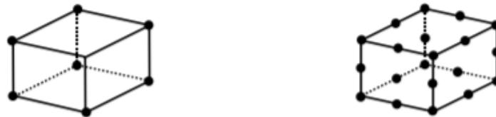
**Figure 19:** Examples of linear (left) and quadratic (right) elements.
