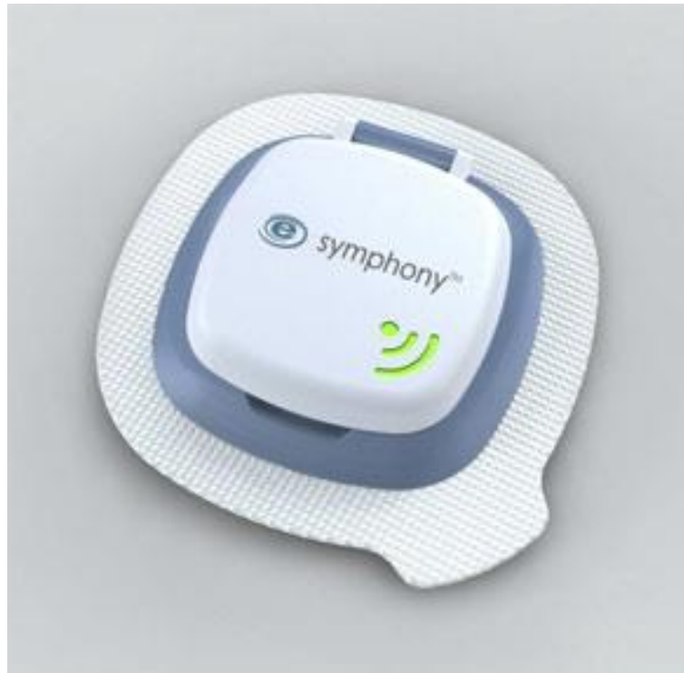
Figure 2-6 Optical glucose biosensor device by Echo Therapeutics Inc (Hoskins, Non-Invasive Diabetes Technology: Still Dreaming, 2012)
