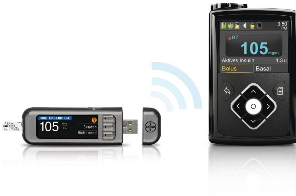
Figure 2-15 Contour Next USB by Bayer constitutes an example of commercial glucose monitoring device having USB (Medtronic - Minimed Product, 2016)
