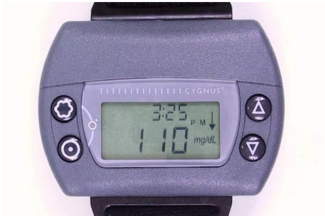
Figure 2-14 GlucoWatch by Cygnus constitutes an example of a wearable glucose biosensor system (Endotext, 2013)
