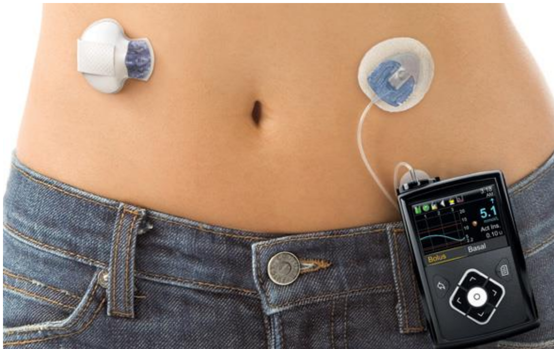
Figure 2-13 Blood glucose biosensor connected to insulin pump (Medtronic, 2016)
