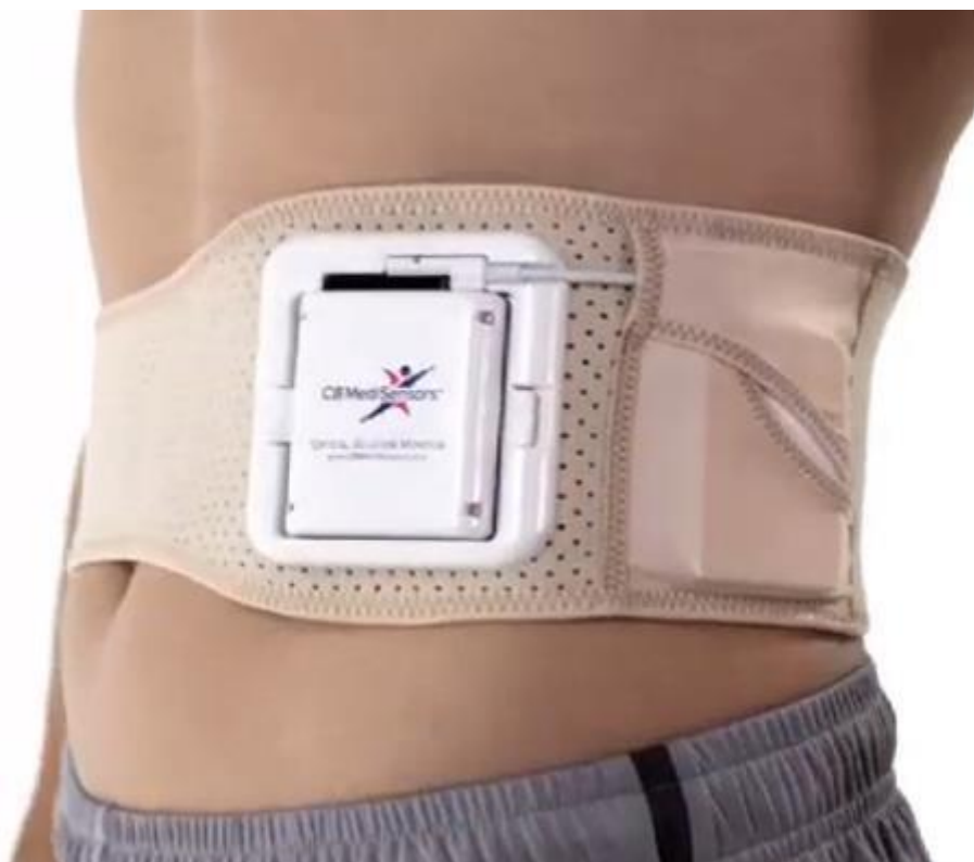
Figure 2-7 Optical glucose biosensor by C8 Medisensors (Napodano, 2013).
