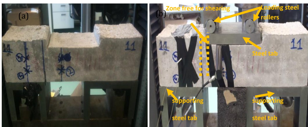
Figure 3.2. 2 (a) Concrete beam with reduced cross section for shear testing, (b) test set up for the shear testing.
