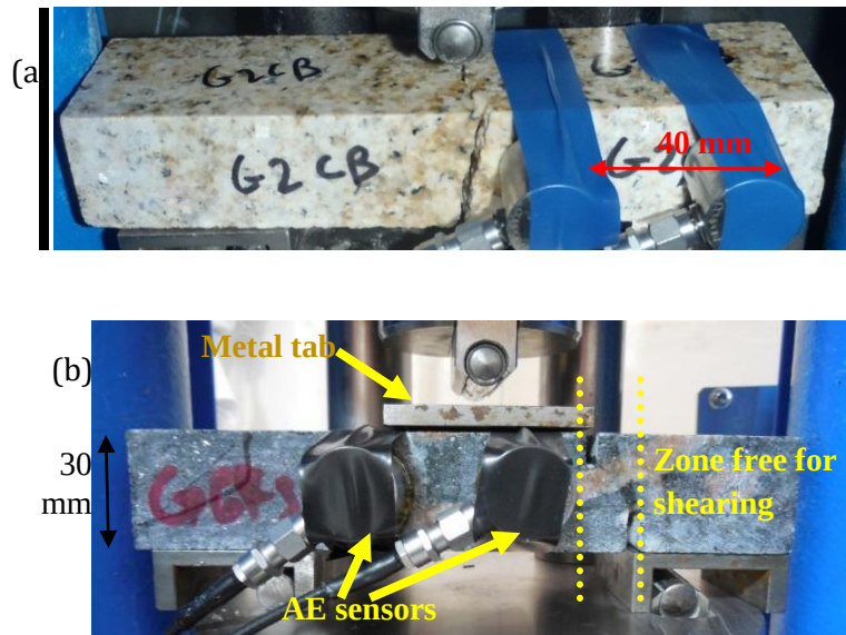
Figure 3.5. 1 (a) Three point bending and (b) shear test of granite with concurrent AE monitoring by two sensors.
