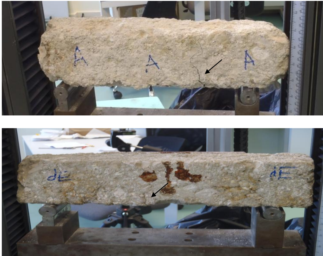
Figure 6. 5 Bending specimen after the four-point bending test. A large crack is visible (see arrow).
