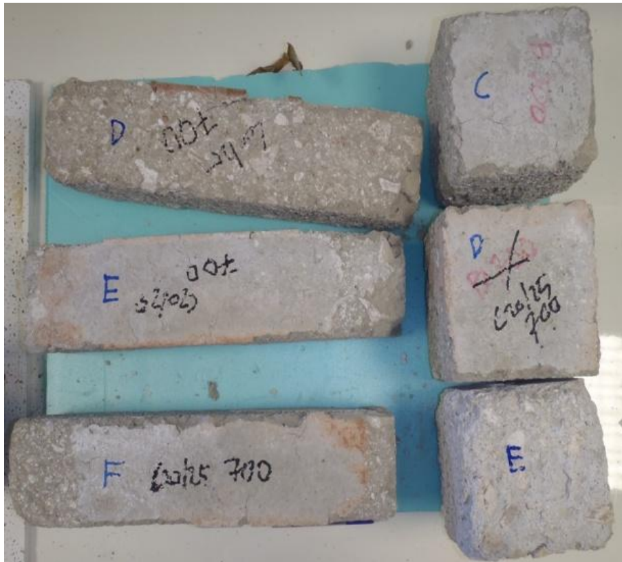
Figure 6. 1 Typical specimens after fire exposure.
